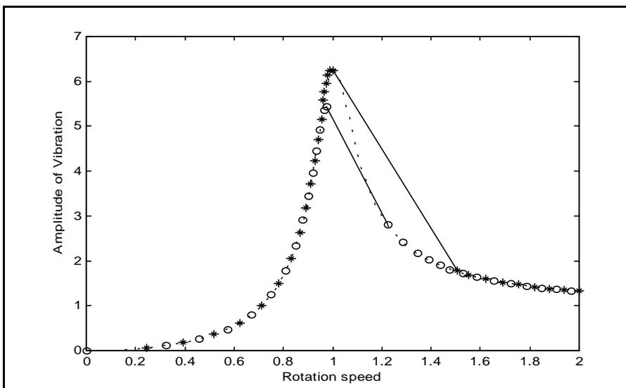
Fig 09 - Vibration amplitude vs. rotation speed. \*: Increasing voltage o: Decreasing voltage
