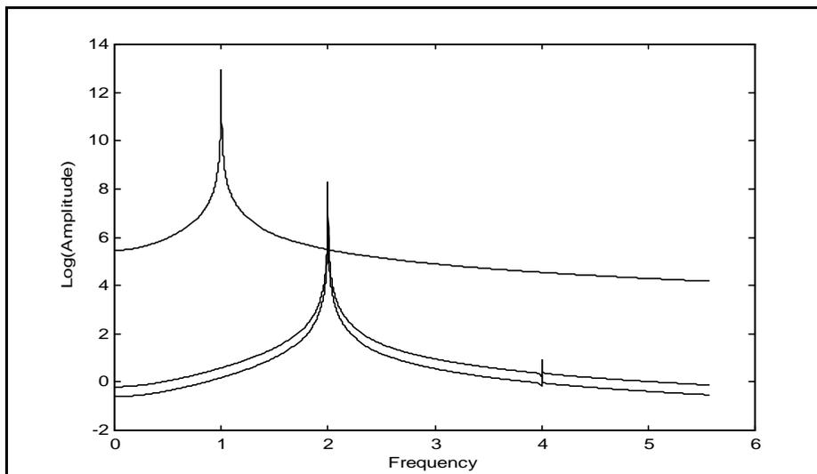
Fig 12 - Spectra for hardening cubic stiffness and null gravity vibration of the table, rotation of the shaft and demanded current (up to down)
