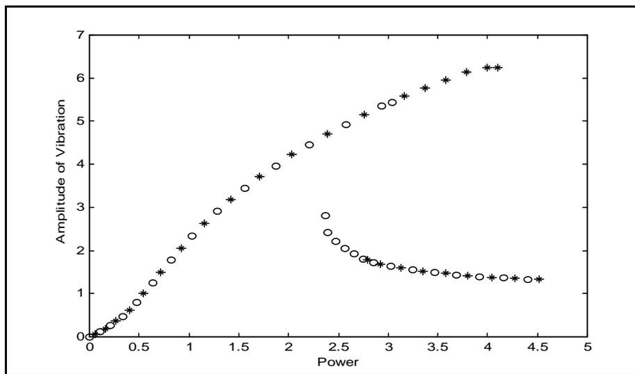
Fig 11 - Vibration amplitude vs. power supplied. \*: Increasing power o: Decreasing power
