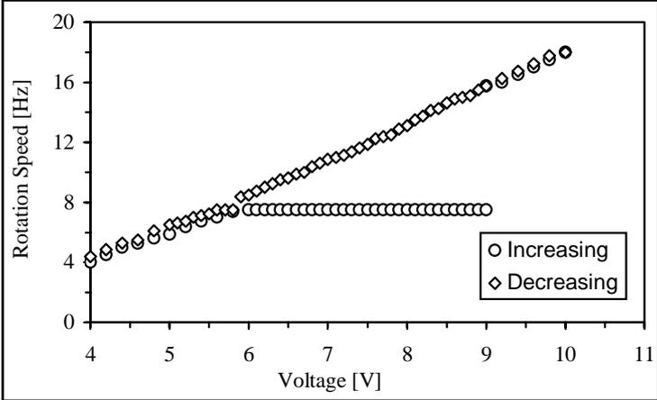
Fig 03 - Rotation speed of the motor vs. applied voltage
