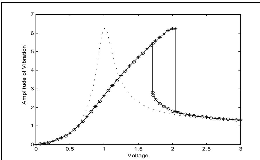
Fig 08 - Vibration Amplitude vs. applied voltage \*: Increasing voltage o: Decreasing voltage
