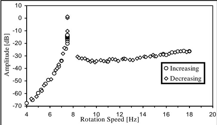
Fig 05 - Amplitude of the first harmonic vs. rotation speed of the motor
