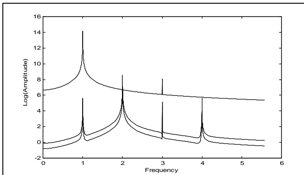
*Fig 13 - Spectra for hardening stiffness and non-zero gravity vibration of the table, rotation of the shaft and demanded current (up to down)*
