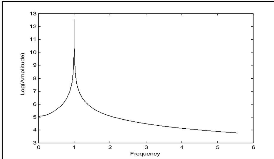
Fig 10 - Spectrum of the response of the beam near the resonance (simulation)
