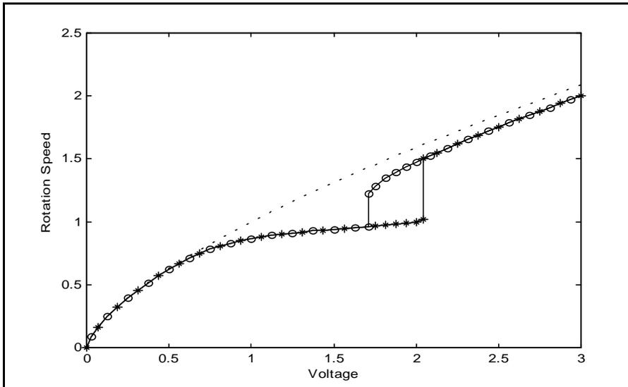
Fig 07 - Rotation speed vs. applied voltage. \*: Increasing voltage o: Decreasing voltage
