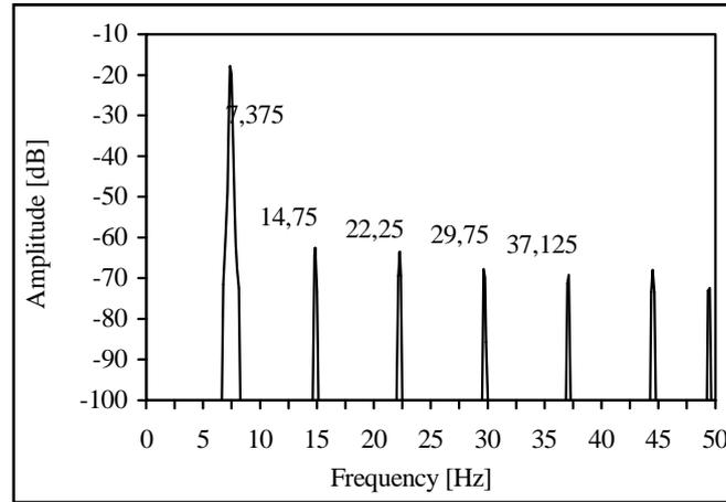
Fig 06 - Spectrum of the response of the system vs. rotation speed of the motor
